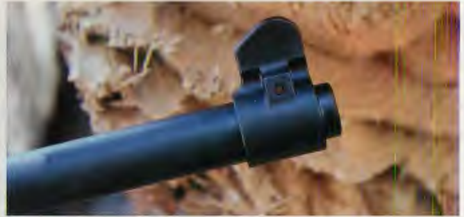
The MOA Mini-14's new rear sight (left) retains a military look and the peep aperture is adjustable for W/E. The new Mini-14 front sight is protected by two ears like that of the M14 rifle. The real news, however, is greatly improved accuracy due to now using hammer-forged barrels.
